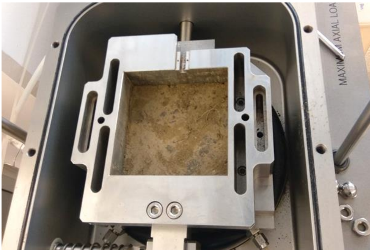
Figure 88: Undisturbed specimen used in the wetting tests installed into the UGDSBPS apparatus at a natural water content.
