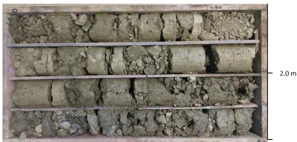
Figure 9: Core samples obtained by machine-drilling at the B1 location with marked depths.
