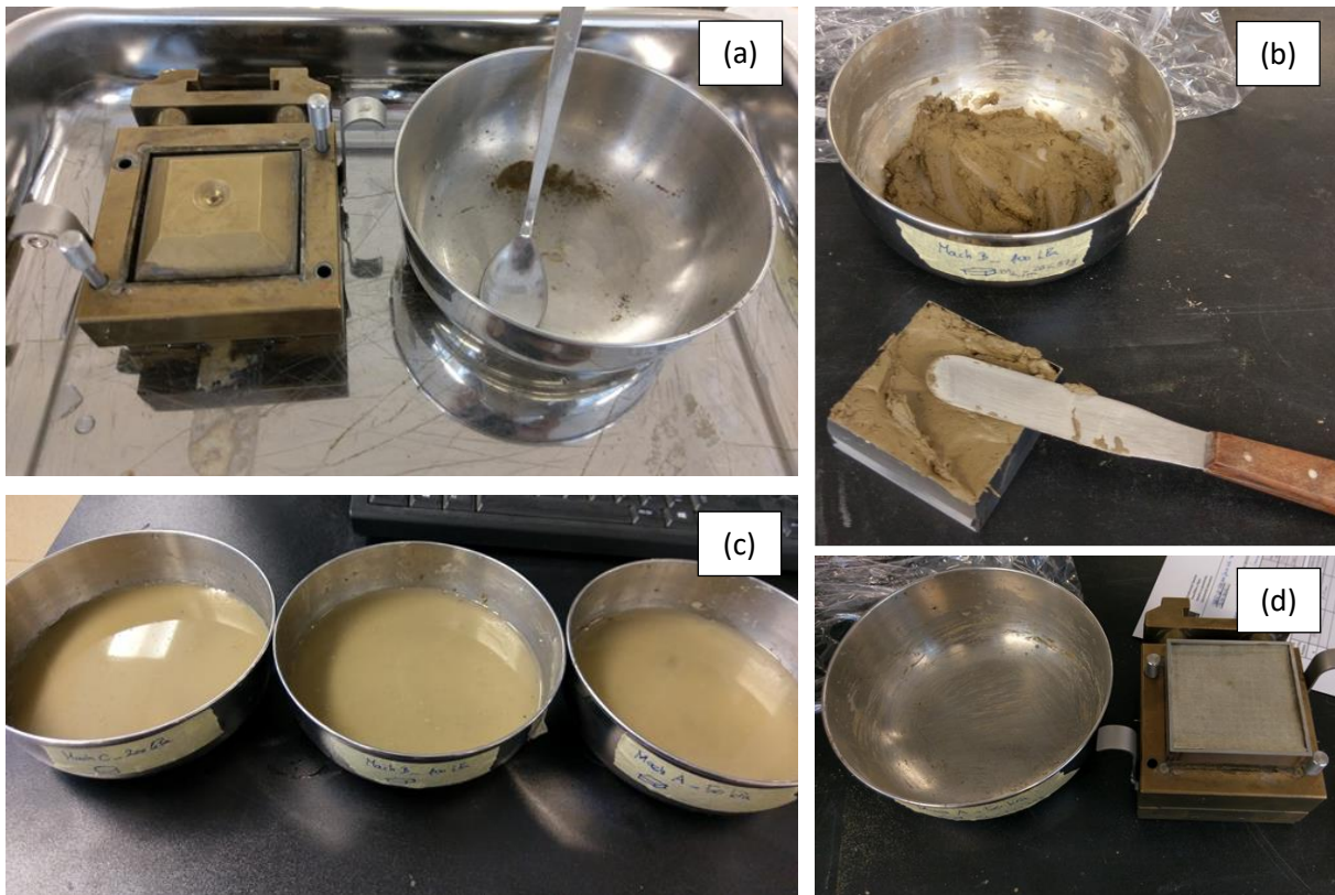
Figure 69: Details of the adopted specimen preparation technique: a) collection of the material after testing the undisturbed specimen for water content determination; b) material thoroughly mixed with de-aired water left to rest over-night; c) installation of sample inside the square cutter; and d) remolded specimen ready for the installation in direct shear apparatus.
