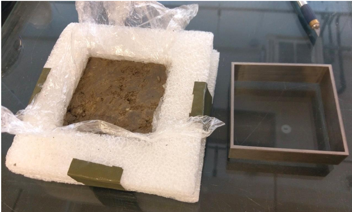
Figure 83: Preparation of undisturbed specimen for testing in the UGDSBPS collected in-situ with dimensions 100x100x20 mm.
