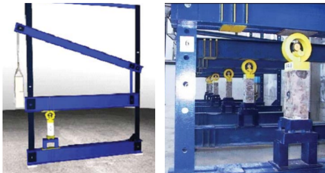
Figure 3.8 Devices for uniaxial creep tests (Tomanović, 2009)
