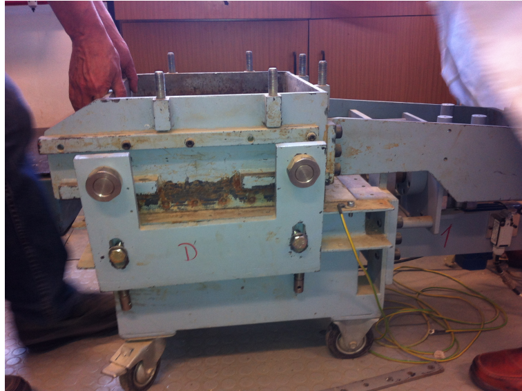
FIGURE 4.8: Large direct shear box at CEI
