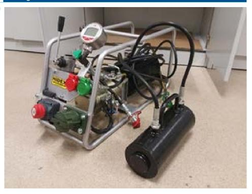
Short description Portable hydraulic device for applying force - MATEST S222-01, S226-1, C405-15, S224-21, S226-05, S226-06 Main purpose Portable hydraulic device for applying force. Technical specification ■ Capacity 100 kN ■ Small hydraulic aggregate 12V DC Source of funding "Research Infrastructure for Campus-based Laboratories at the University of Rijeka" project financed by ERDF Contacts Davor Grandić / dgrandic@uniri.hr
