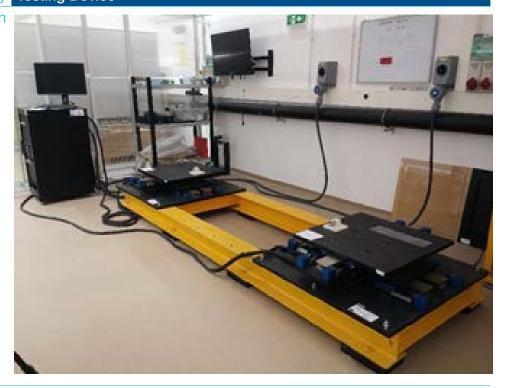
Short description System of two biaxial shaking tables Quanser STI-III actuated by electromagnet motors (control unit, hardware + software)
