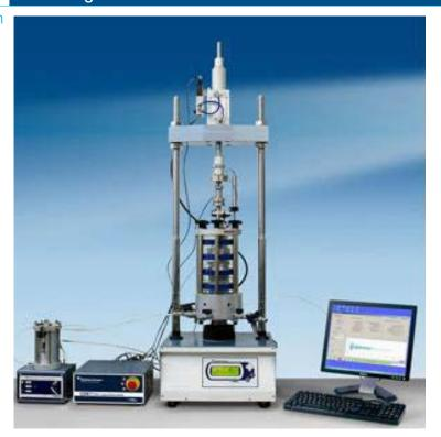
Short description Contains: cell for triaxial test with dynamical/cyclic load, LVDT, measuring cell and pressure transducers. Depending on the sample size, triaxial cell can be changed. Possibility of testing samples of diameter: 38, 50 and 70 mm. Can simulate earthquake accelerations.
