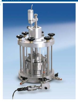
Short description Inner cell contains sample, outer cell used for loading, ring for sample preparation, LVDT with pressure transducers.
