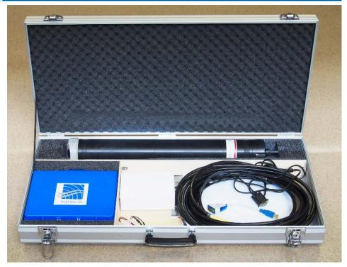
Short description ADCP allows measurements of characteristics of sea currents.
