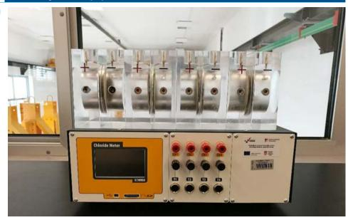
Short description Chloride penetration meter is used for measuring the electrical resistance of concrete against the penetration of chloride according to the standard methods. The test device is equipped with 4 independent channels and 4 test cells suitable to perform tests on up to 4 specimens. Equipped with vacuum saturation apparatus necessary to fully saturate the specimen with water.
