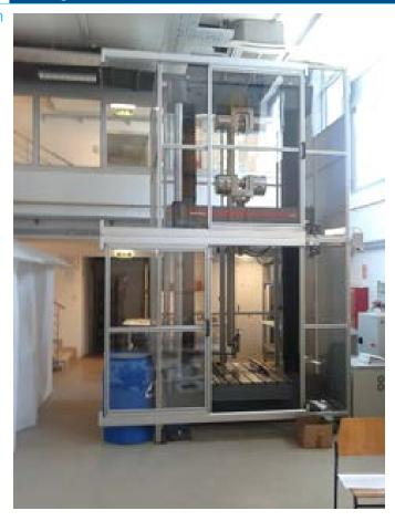
Short description Universal tension-compression testing machine Zwick Z 600E with capacity 600 kN and electro-mechanical drive. Testing machine consists of two workspaces. The upper workspace is primarily designed for tensile tests, while the lower working space is designed for compression and bending tests.
