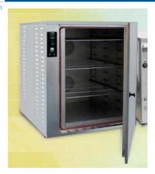
Short description Machine used for drying material. It consists of three grid shelves, cooling fan and temperature gauge.
