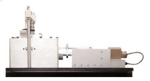
Short description Device consists of external hydraulic unit for controlling the pressure in the chamber, central control unit, servo pump for obtaining internal strain in the sample and bender elements.
