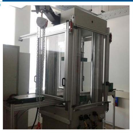
Short description Hydraulic unit, triaxial cell, sample stand, sample deformation gauges, uniaxial strength and tensile strength adapters.
