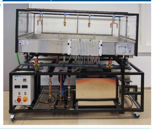
Short description The advanced hydrological test chamber is equipped with 8 nozzles that can be used to model various hydrological conditions.
