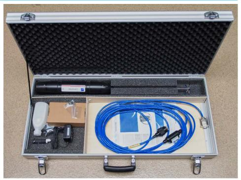
Short description Vectrino profiler is used for measurement the velocity vector along a water column with length between of 0.5 m to 3 cm.
