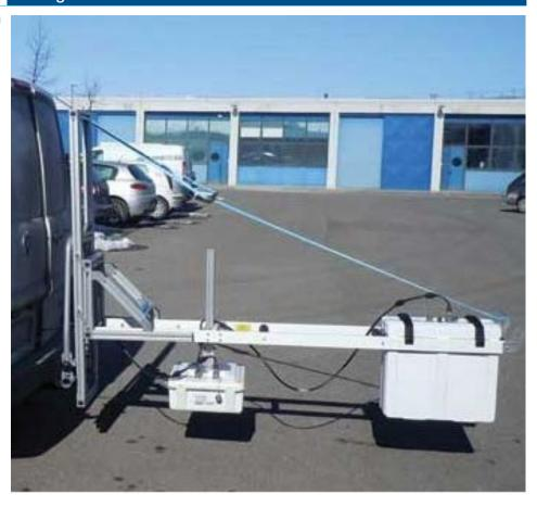
Short description Antenna 2 GHz and dual frequency antenna 400-900 MHz. High speed survey wheel for distance measurement, mechanical frame to install system on vehicle and PC for data aquisition.
