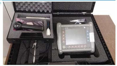
Short description Portable combined hardness tester for steel MIC 20 TFT (two sets of probe, cables, software)
