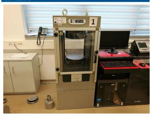
Short description The servo-hydraulic compression frame 3000 kN capacity can be used to perform various building material tests. It is suitable for testing cubes up to 200 mm and cylinders up to diameter 160 x 320 mm. The frame is completed with suitable distance pieces conforming to the specimen size .
