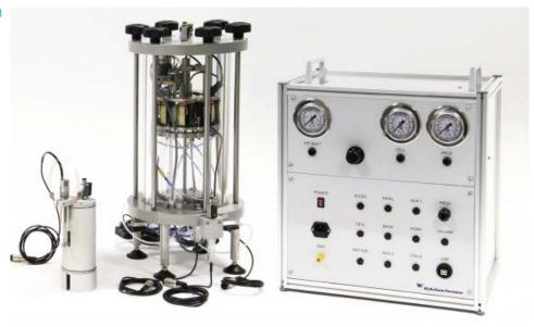
Short description Device for testing resonant characteristics of fine grained soil. Pedastel for 50mm sample, LVDT, brass and steel calibration rod
