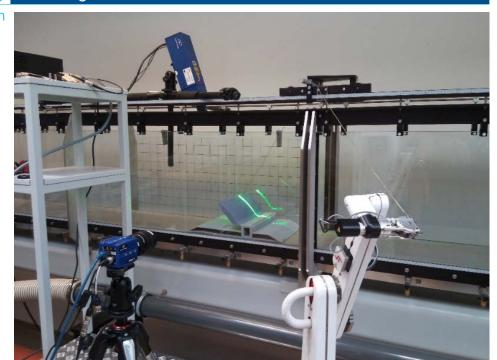
Short description The synchronized high-speed camera and laser assembly allows the reconstruction of the flow field in a flow plane.
