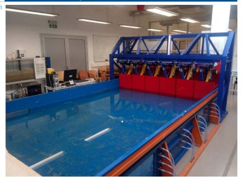
Short description Experimental pool with a wave generator for testing of physical models of naval construction and deformation of waves. The experimental pool offers also the possibility of modeling ocean currents.
