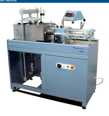
Short description Machine used for direct shear of samples dimensions 30 x 30 cm. LVDT: horizontal and vertical, shear platen used for better grip sample. Main purpose Determination of shear strength of coarse-grained soil.
