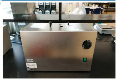
Short description The internal chamber and the insulated exterior case of the bath are manufactured from stainless steel. It has timer which is used to set the time for reaching the boiling point in 30 minutes by using two heater units. The bath is supplied complete with a 12 place Le Chatelier mould rack.
