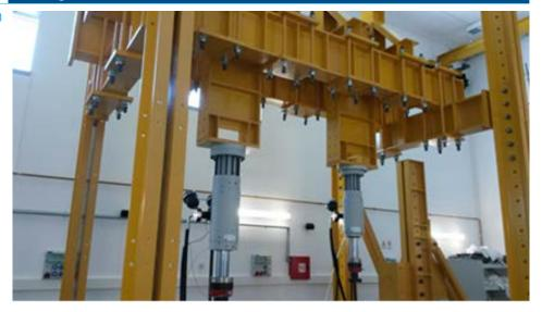
Short description Dimension of steel load frame 5,0 x 3,6 m, has the possibility of extending to 7,0 m in the longitudinal direction and to 6,0 m in height. Capacity of actuators are 500 kN and 250 kN. Actuators have been specially designed for dynamic material testing for determining the fatigue strength of material and components of structure. The entire system is controlled via a computer program Cubus.
