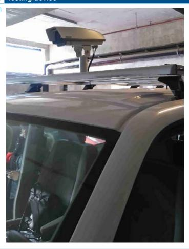
Short description Video camera in waterproof enclosure connected with laser profiler measure-
