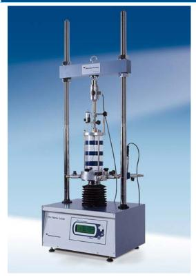
Short description Triaxial cell. Consists of: LVDT, measuring cell, pressure transducers. Triaxial cell can be changed depending on the sample size. Possibility of using benders and on-sample transducers.
