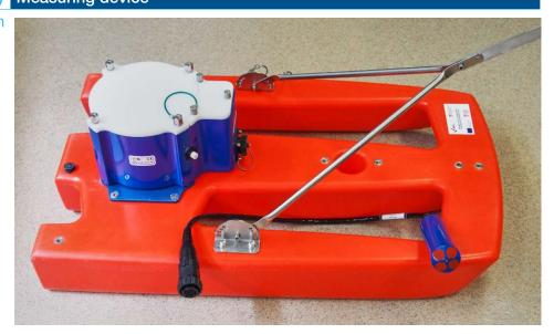
Short description ADCP is designed for surface recording of flow characteristics in rivers and lakes.
