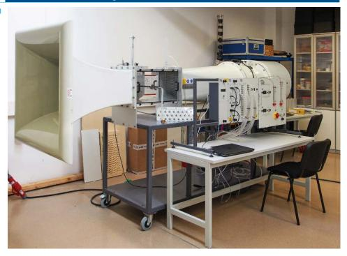
Short description Wind tunnel for testing aerodynamic characteristics of different physical models.
