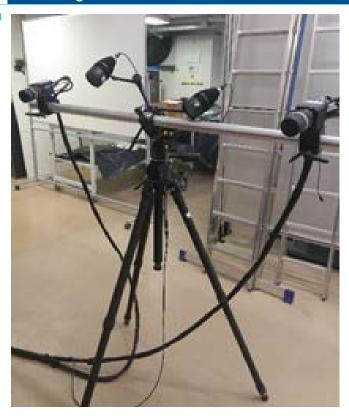
Short description Optical measuring system GOM mbH PONTOS 3D 4M: head with two cameras, cables, support, calibration object, lenses, laser pointer, LED lights, cases
